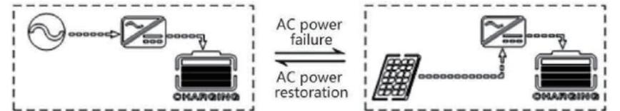
**3. Mixed charge:** with mixed charge through photovoltaics and mains supply, photovoltaic MPPT charge is used preferentially. In case of insufficient photovoltaic energy, the mains supply is used for supplement. In case of sufficient photovoltaic energy, mains supply stops charge. Electricity can be charged fastest with the way, which is suitable for the area with unstable power grid, so as to supply sufficient backup power supply at any time.
