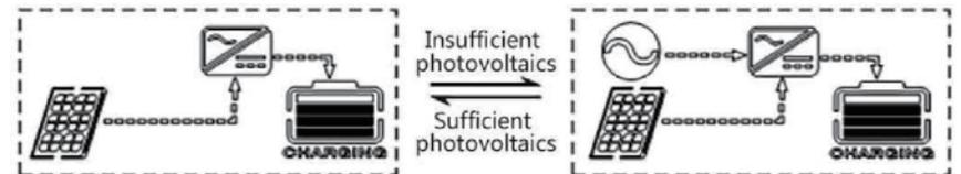
**4. Only solar:** only photovoltaic charge is used, no mains supply is started. This way can save the energy at most. The electric energies of battery are all from solar energy. This way is suitable for areas with good light condition.
