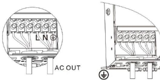
**Note:** use thick ground cable as far as possible (with cable section not less than 4mm<sup>2</sup>), place the ground point to be close to the all-in-one machine as far as possible and choose shorter ground wire to the greatest extent
