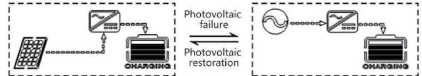
**2. Mains supply priority:** mains supply is to charge the battery preferentially and the photovoltaic charge can be started only when the mains supply is valid.
