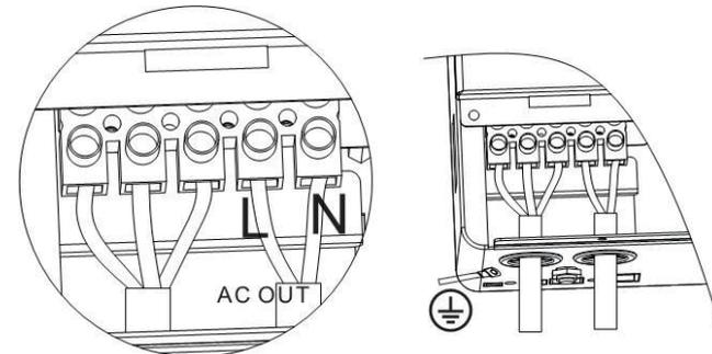
**Note:** The grounding wire shall be as thick as possible (cross-sectional area is not less than 4mm<sup>2</sup>). The grounding point shall be as close as possible to the all-in-one solar charge inverter. The shorter the grounding wire, the better.
