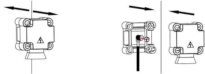
**Note:** Press the position indicated in the figure above before disconnecting the power terminal.
