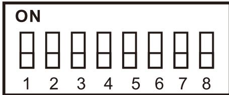
**DIP switches definition:** Bit1~Bit5 is used to set the slave address or the number of slave parallels according to the host and slave status. Bit6 is used to set the host and slave flags.
