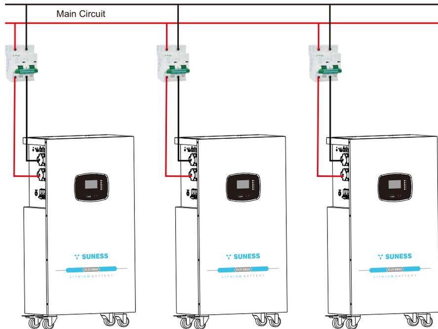
**Step 1:** The parallel connection of three battery packs is presented in Figure 1.
