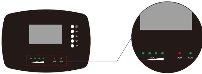
The BMS features 6 external LED indicator lights. 1. 4 white-green capacity indicator lights. 2. 1 red alarm indicator light. 3. 1 white-green operational indicator
